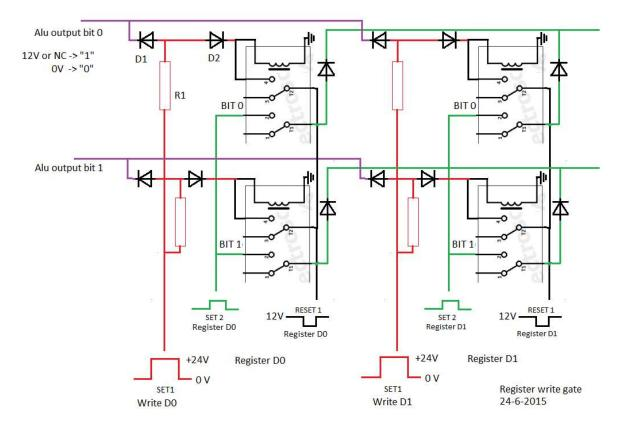
The output of the ALU is connected to several registers. We need a method to write this output to a certain register without affecting the contents of the other registers.
