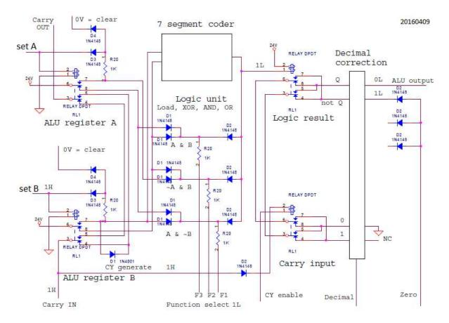
In the schematic, codes are used: OL means logic "O" is connect to low voltage level (pulldown to ground), 1L means logic "1" is pulldown to ground, 1H means logic "1" is connect to high voltage (pull up to 12V or 24V).
