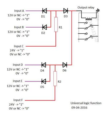
The AND function can be combined with an OR function. The circuit above shows two 3-input AND gates, the outputs of the AND gates are inputs to a 2-input OR gate (built with D3 and D6). It gives the following logic function:
