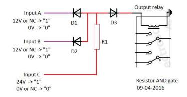
In the following parts of this story, it is supposed that 12 Volt relays are used and that the resistors have the same resistance as the relay.
