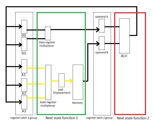
This diagram shows the most important parts of the CPU. It has the following functionality:
