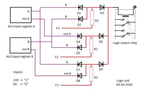
The next diagram shows the logic functions of the ALU (only a single bit shown):
