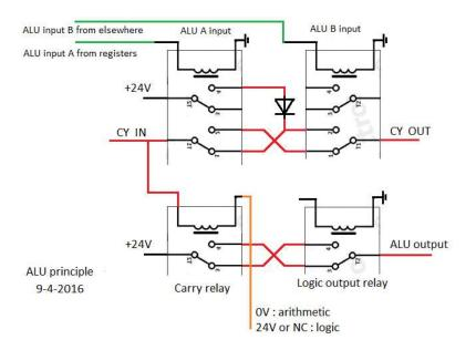
The logic output relay is added to the diagram. The input circuit to this relay is not shown here, but is comparable to the logic function unit. discussed before.
